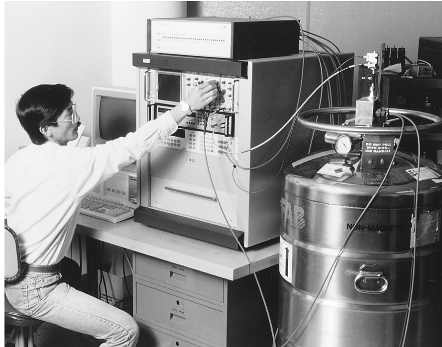
The Fluke Standards Laboratory offers traceability to its own 10V Josephson Array, an intrinsic standard of voltage, and to national standards.
